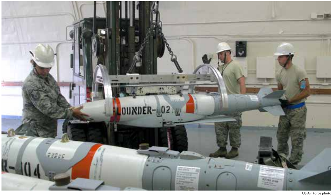
Figure 2. Airmen from the 36th Munitions Squadron load a recently assembled Quickstrike-ER onto a munitions trailer.
